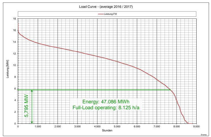
⇒ Preheating with DLK4 result in 47.086 MWh/a energy savings (process stream)
