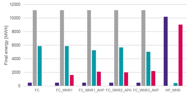
Results of simulations for 1MW of IT equipment in the data centre.
